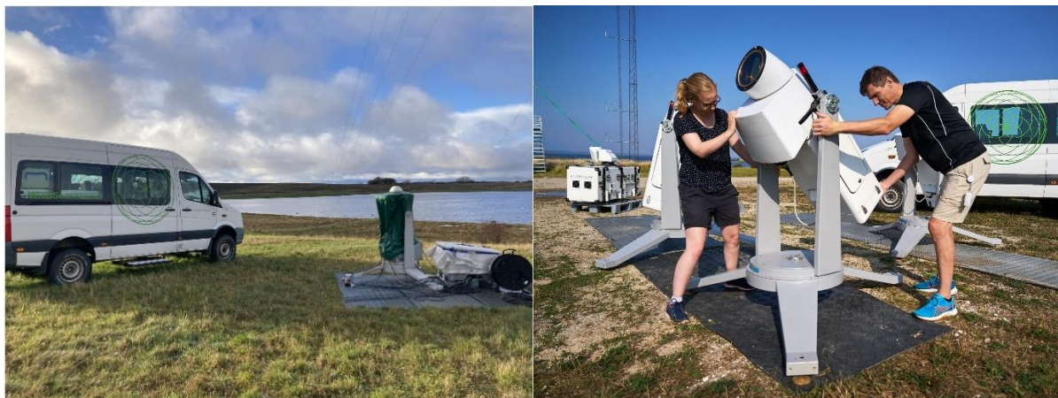
Figure 1 – The continuous-wave laser-based short-range WindScanners developed at DTU Wind.
